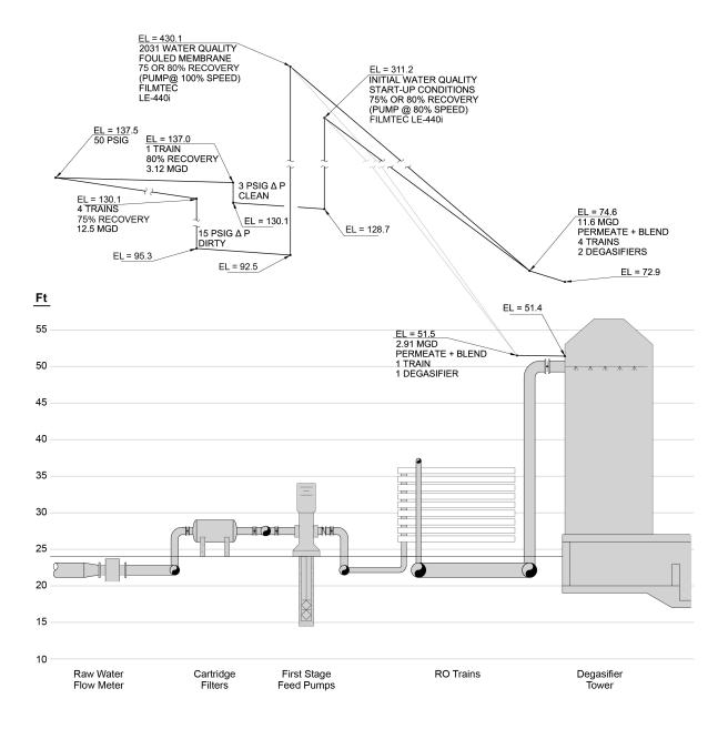
Figure 3-3. Sample hydraulic profile – membrane feed and permeate.
