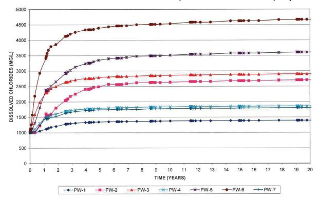
Figure 3-1. Projected dissolved chloride variations at brackish well field.
