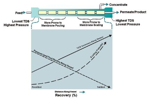
Figure 3-5. Flux decline within a pressure vessel.
